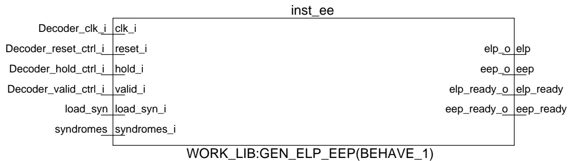
Figure 18: Block diagram of the ELP and EEP computation block
